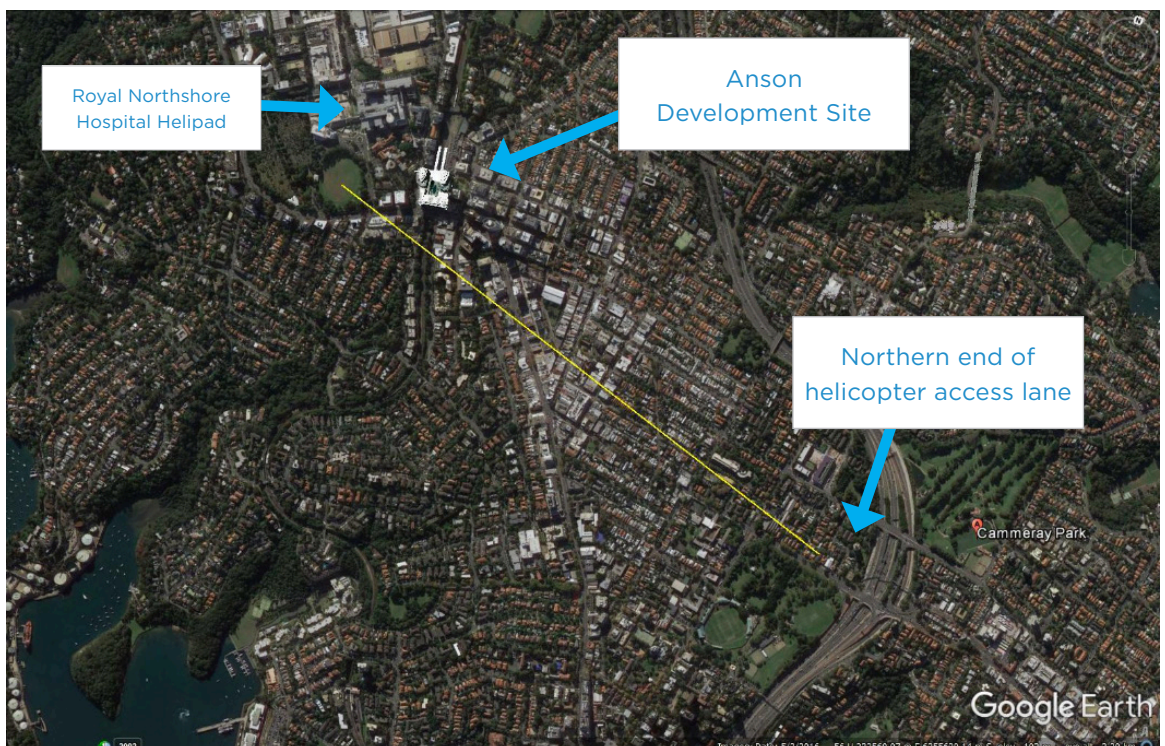
Figure 9: RNSH Helipad preferred approach point from end of helicopter access lane
